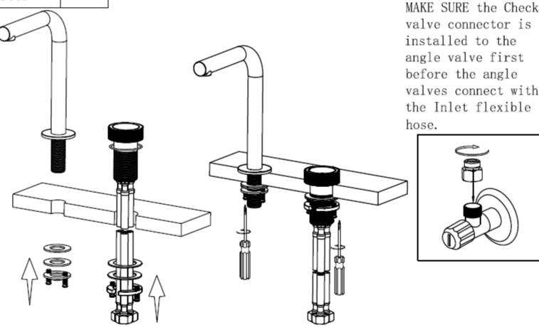
4. Screw out and take off the nut, rubber washer and metal washer from the spout. Put the spout into the hole of  $\phi 23$ mm on the counter and screw up the nut, rubber washer and metal washer again to the spout, and fix it on the counter by tightening the screws on the nut with screwdriver.
