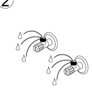
Fush any contaminates in supply lines for 30~60 seconds until water is clean.
