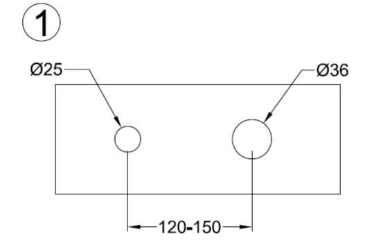
1.Make two holes with a proper center distance of 120~150mm on the counter, with the left hole having a diameter of 23mm and the right hole of 38mm.
