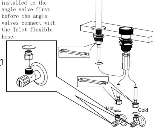
5.Connect the Outlet flexible hose(5) to the spout(1). Install the Check valve connector(9) to angle valves linked with Hot & Cold water supply pipe, then fasten it by spanner to the other end of the Inlet flexible hose(Red for hot, Bule for cold)(4).(All done)
