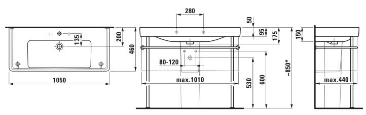
\* = Effective height must be fixed according to the height of the pedestal.
